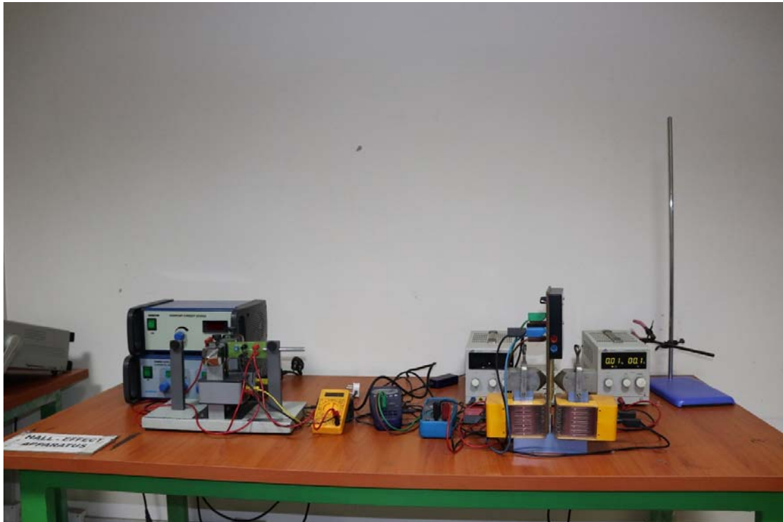
Hall effect measurement system at research level for quantifying charge carriers' concentration
