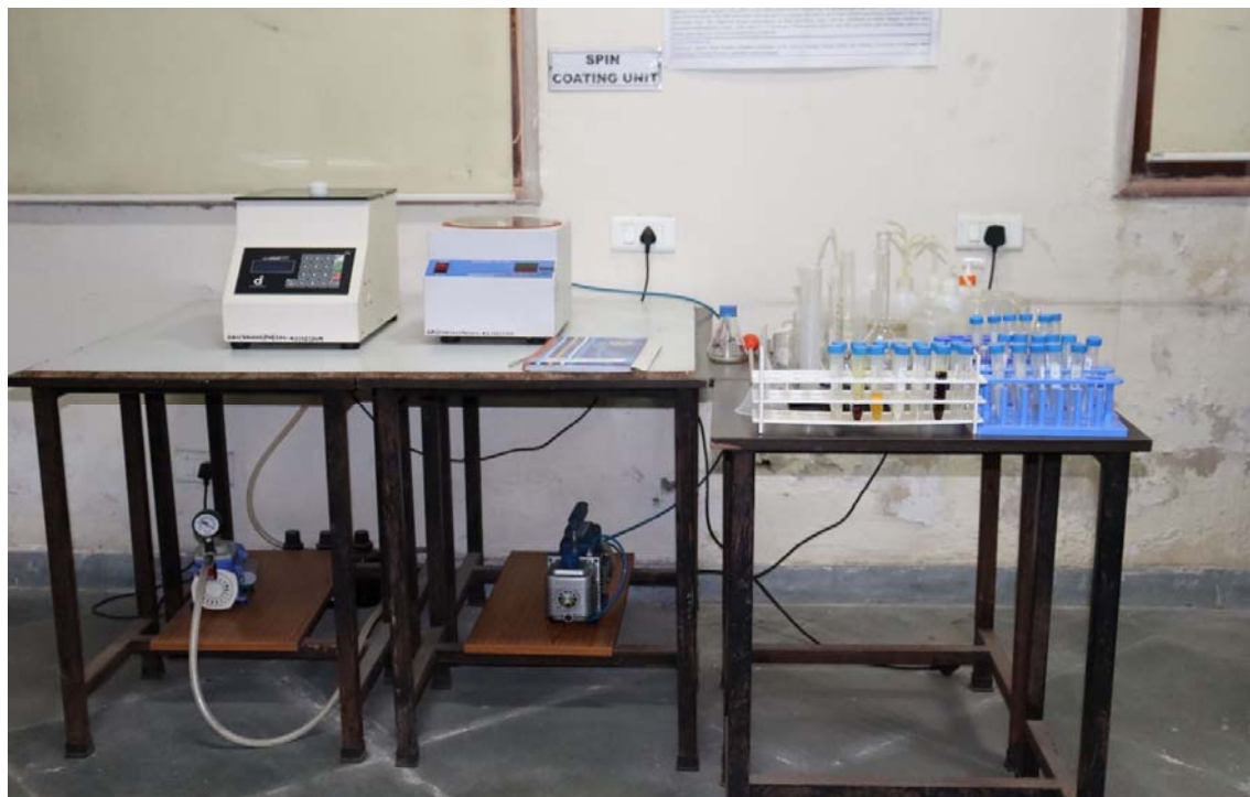
Thin film deposition by spin coating
