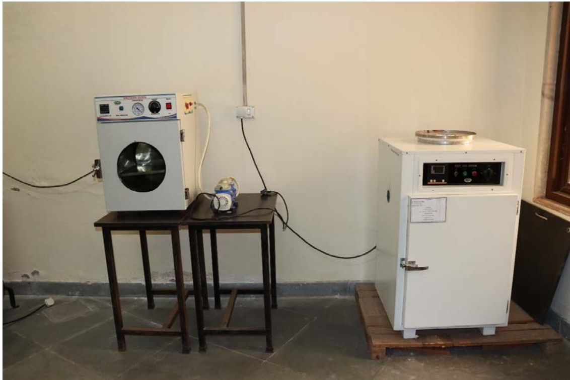
Furnace and oven for thermal treatment of materials and micro samples synthesis by solid state diffusion
