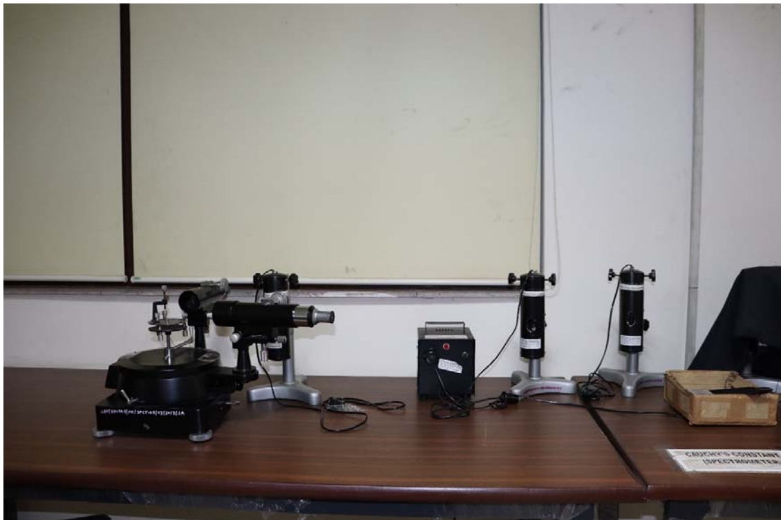
Manually controlled spectrometer for rough testing of materials
