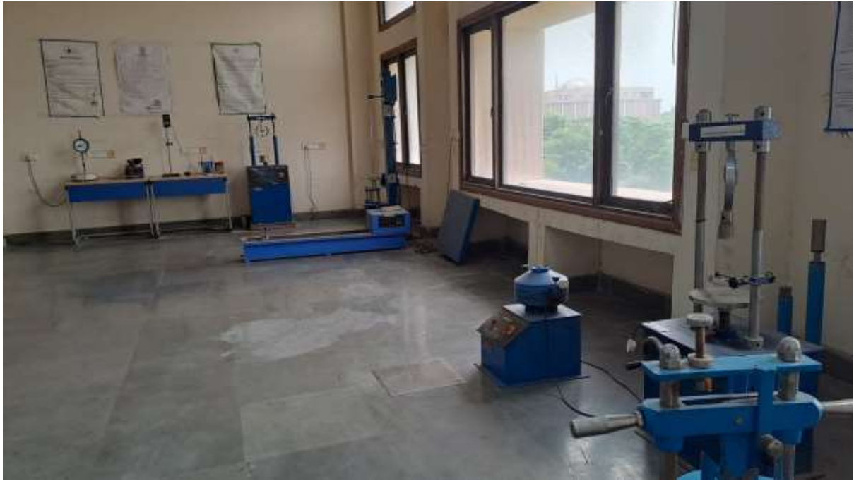
Transportation lab for the study of impact test of coarse aggregate, CBR value, penetration, ductility, flash and fire point, softening point for bitumen.
