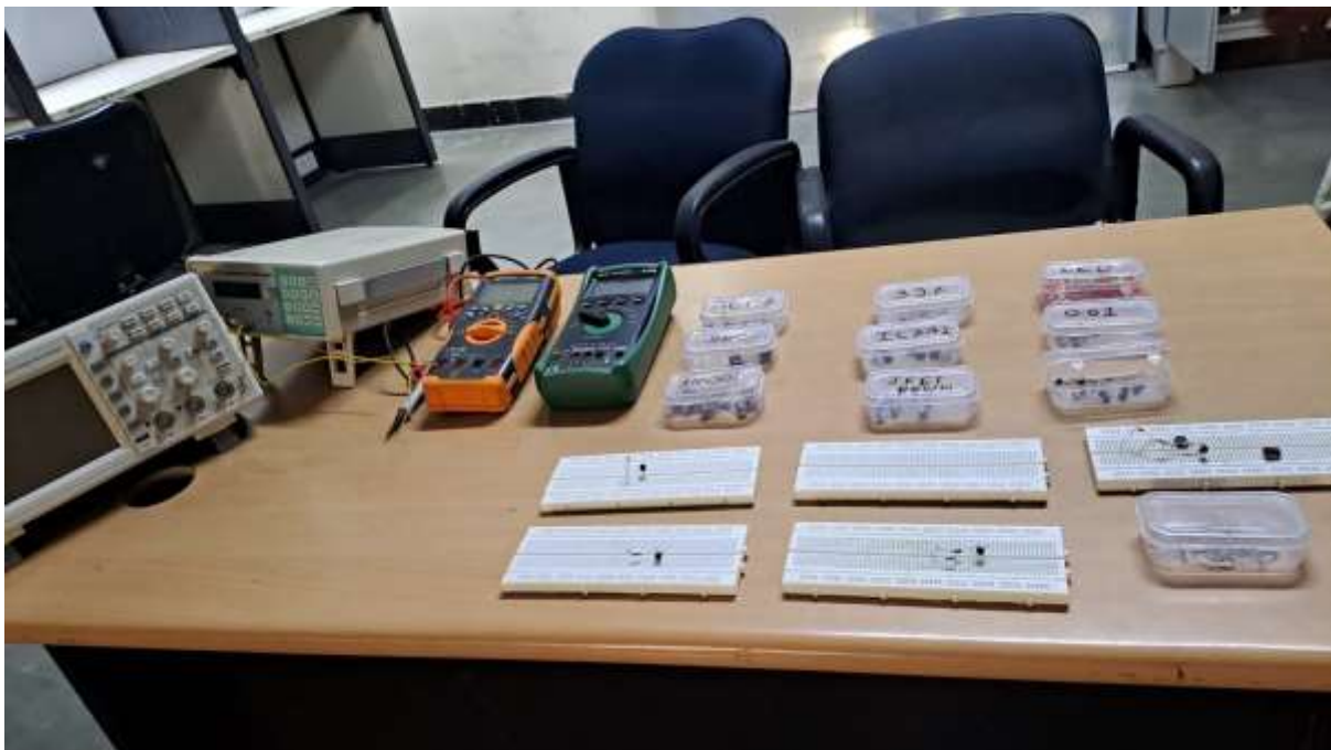
Electronics device and circuit lab for the study of switching action of a transistor, op-amp as inverting amplifier, non-inverting amplifier, differentiating amplifier, etc.
