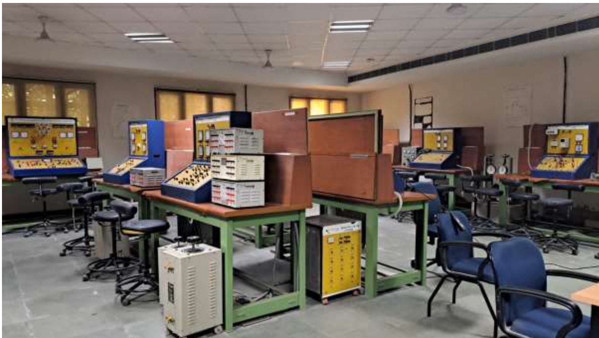
Electrical machine lab for the study of polarity and ratio test of single phase and 3-phase transformer, open circuit and short circuit test, efficiency and voltage regulation, DC compound motor, DC shunted and series motor, etc.
