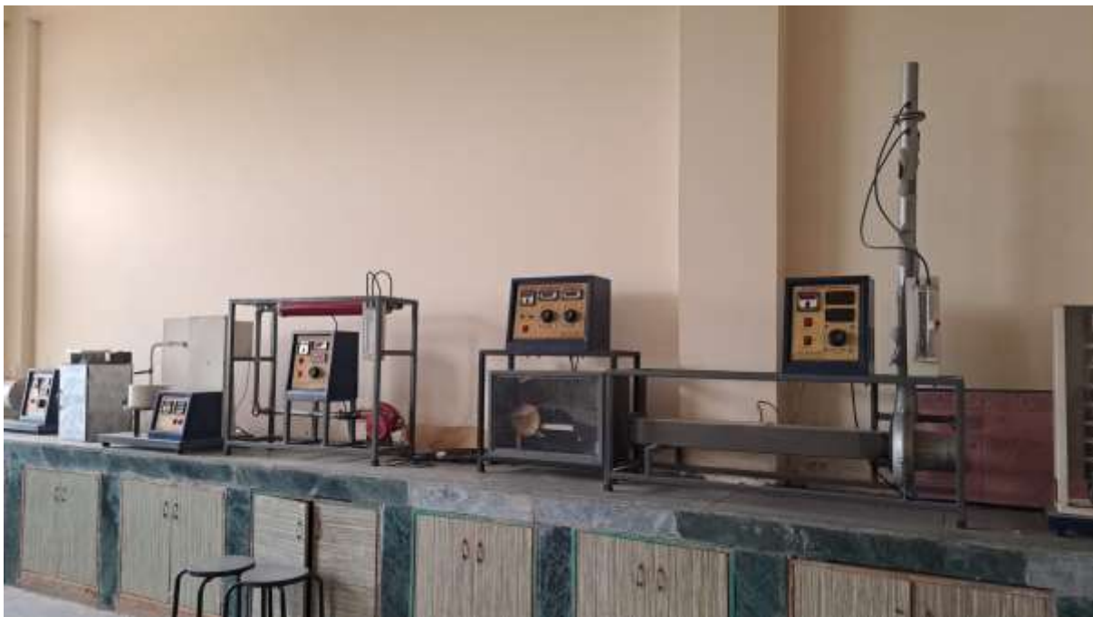
Heat and mass transfer lab for measurement of thermal conductivity of powder, emissivity, forced convection, thermal conductivity of liquid and study of Stefan-Boltzmann apparatus.
